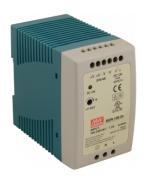
The AC/DC switching power supply is intended for supplying devices requiring a DC voltage of 24V and a total efficiency of 4A @ 24V DC. It has the following protections: short circuit (SCP), overload (OLP), overvoltage and overheating (OHP). The power supply is housed in a housing adapted for mounting on a DIN rail.
