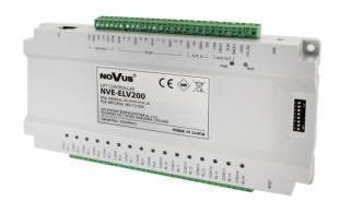
The lift controller realizes centralized management by connecting indoor monitor, outdoor panel and Wiegand card reader. With easy operation and setting, this device meets users' diversified needs. The module has two operating modes. The module relays can be connected directly to the elevator buttons or to the PLC inputs. Lift controller can be set to master and slave types. In one lift controller unit, the Master Controller communicates with other slave lift controller by RS485.
