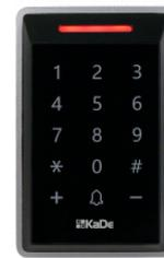
The KDH-KZ3000-IP-U\_M controller has been designed for access control system and to be mounted on a wall without any additional enclosure. 32 bit processor ensures fast and reliable data processing. This is one door controller. With additional reader (also with keypad) it can use for two way control. It's possibility to set one from four identification mode: Card only (default mode); PIN only; Card or PIN; Card + PIN
