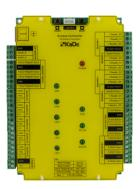
The KDH-KS3024-IP standard controller is designed to work with the new **NOVUS MANAGMENT SYSTEM AC** physical access control system. Communication with the system server is based on TCP/IP protocol via the Ethernet port on the controller board.
