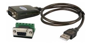
The KDH-USB / RS485 converter is used to connect the controller bus to a USB port on a computer with a supervisory program. The device allows conversion of the USB protocol to RS-485 creating a virtual COM port. The converter has surge protection. The USB port is a cable with a USB connector and the RS-485 port has a DB9-M connector. In addition to the DB9-M connector, you can connect an intermediate module with terminals for bus cables.
