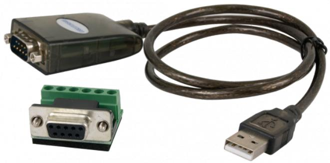
The KDH-USB / RS485 converter is used to connect the controller bus to a USB port on a computer with a supervisory program. The device allows conversion of the USB protocol to RS-485 creating a virtual COM port. The converter has surge protection. The USB port is a cable with a USB connector and the RS-485 port has a DB9-M connector. In addition to the DB9-M connector, you can connect an intermediate module with terminals for bus cables.
