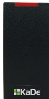
Proximity card readers type KDH-C100H are designed for use in access control systems. Models C100 can be installed inside or outdoors. They have housing made of ABS plastic. The devices reads the HID Prox (125 KHz). The range of the proximity card reading is from 2 to 5 cm depend of the model and type of card.
