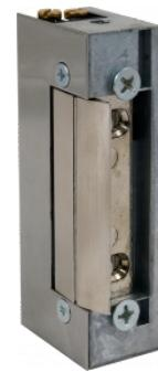
Electric strike (NC), low current. For remote wired opening of doors, gates, flaps, furniture. It can be used in steel, aluminum, wooden and PVC profiles, both internal and external, with the possibility of assembly for left and right doors as well as in vertical and horizontal position. Adjusting the hook in the range of 4mm facilitates assembly and ensures precise adjustment of the electric strike to the handle lock.
